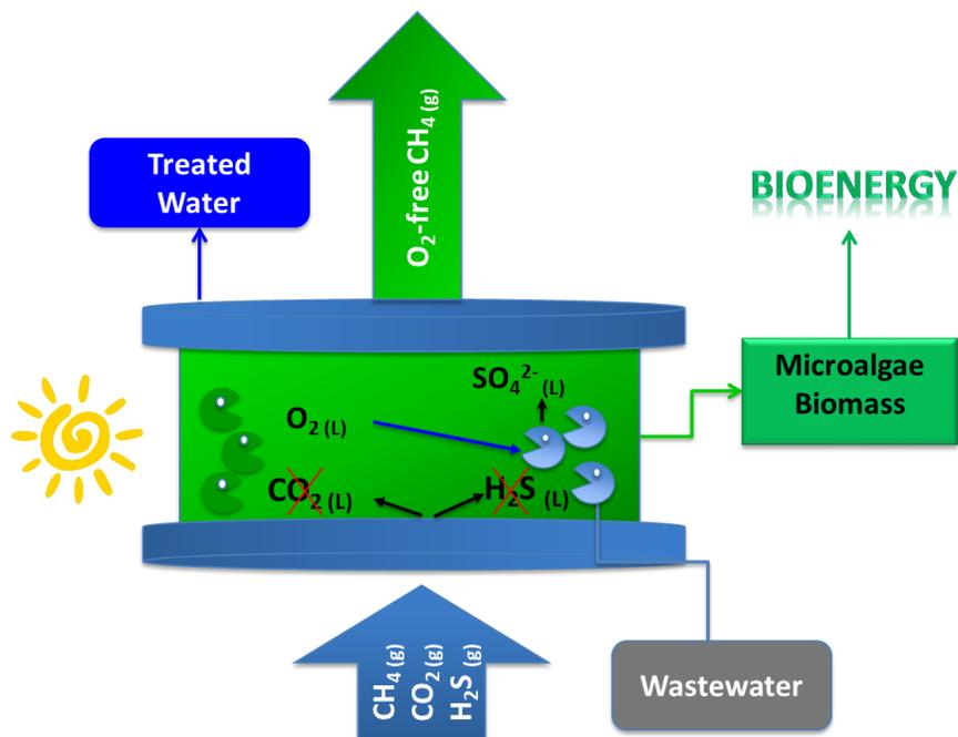
**Figure 1.** Fundamentals of photosynthetic biogas upgrading.
