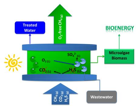
Figure 1. Fundamentals of photosynthetic biogas upgrading.
