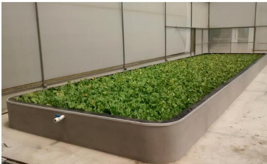
**Figure 1.** A phytofiltration lagoon (13,000 L) with *P. stratiotes* is the first module at INECOL's biorefinery.
